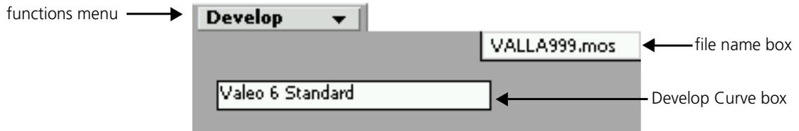
The Develop Curve box displays the develop curve of the selected shoot setup.
