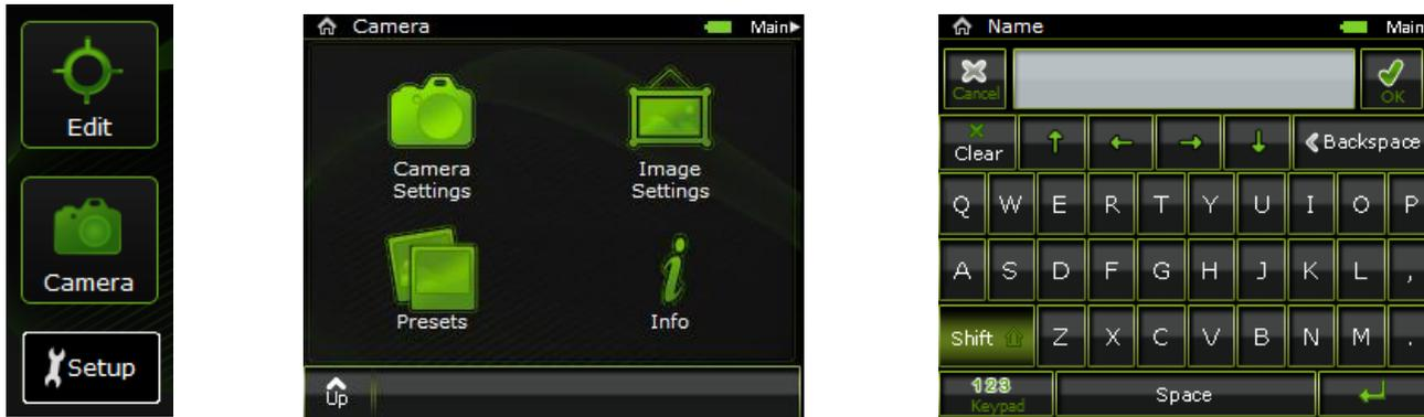
Tap Camera → Camera Settings → Lens → Use the Keypad or Keyboard to enter the Lens Value → Tap OK
