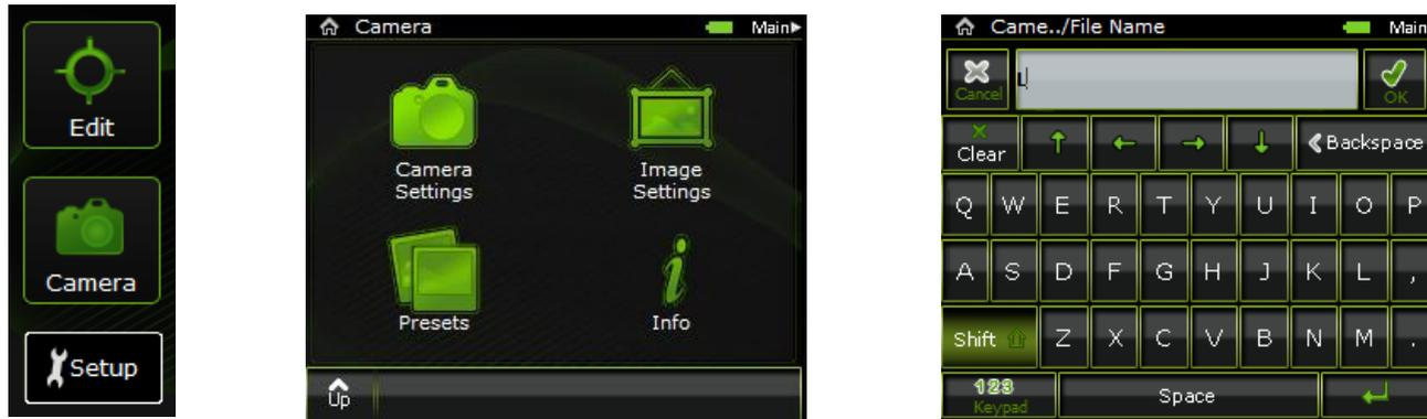
Tap Camera → Camera Settings → Use the Virtual Keypad or Keyboard to enter the desired File name → Tap OK
