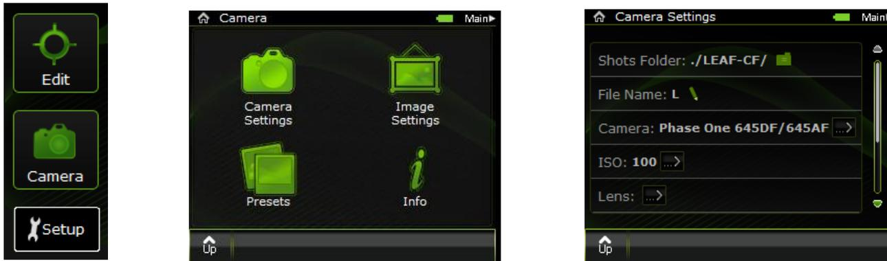
Tap Camera→ Camera Settings→ View the current settings by scrolling up and down.
