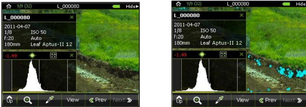
Long tap on displayed image → Tap Over - A flashing mask covers the overexposed and underexposed areas of the image
