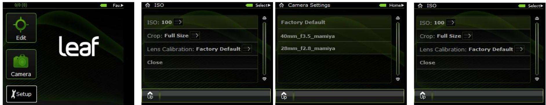
Press ISO button → scroll down to Lens calibration → Press ISO button → scroll and press the desired lens calibration → Scroll with ISO button to Close, and press ISO button.
