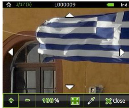
Tap Zoom Button → Tap at the desired position in the image to enlarge by 25% → Keep tapping, directing to the desired area until image is zoomed to 100% for you to check focus.
