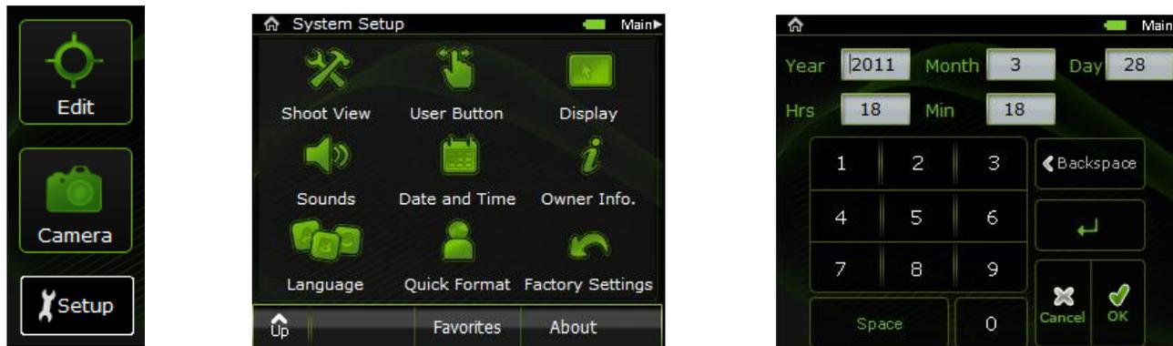
Tap Setup → Date and Time → Use the virtual keypad to tap in the Date and Time → Tap ok
