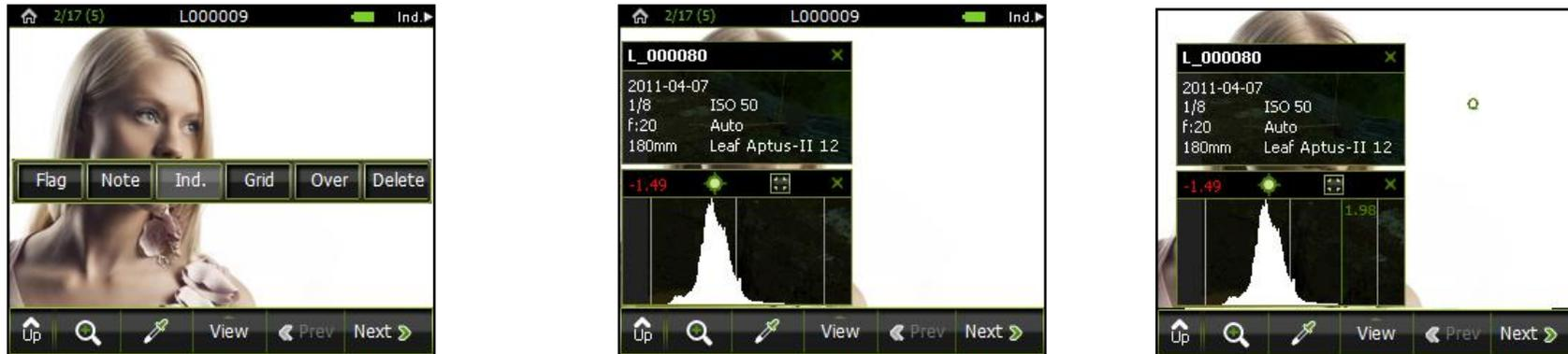
Long tap on displayed image → Ind. OR press User Button → Tap
