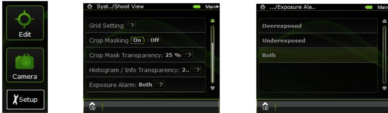
Setup → Tap Shoot View Options → Scroll down to Exposure Alarm → Tap the desired setting
