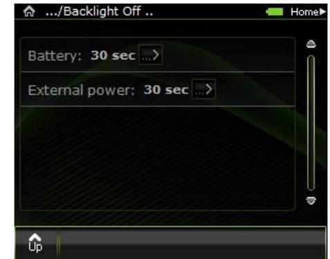
Setup → Tap Display → Backlight Off After → Tap the power source → Tap the desired time
